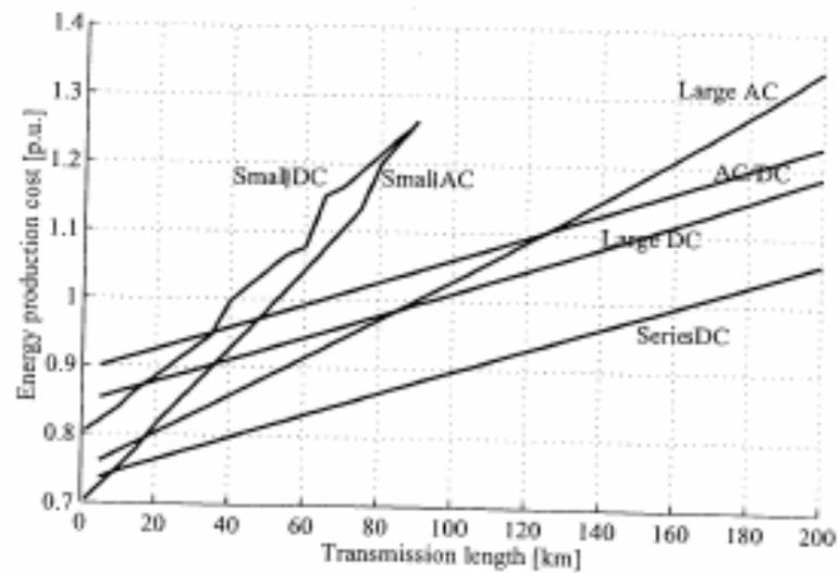
Fig. 3.9 The normalized energy production cost of the different 160 MW wind farms as function of the transmission distance and at a average wind speed of 10 m/s.
